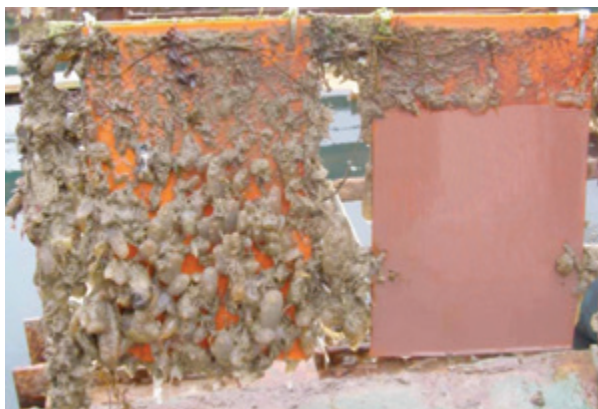
Control and CopperClad-treated sheets after 1 year immersion
